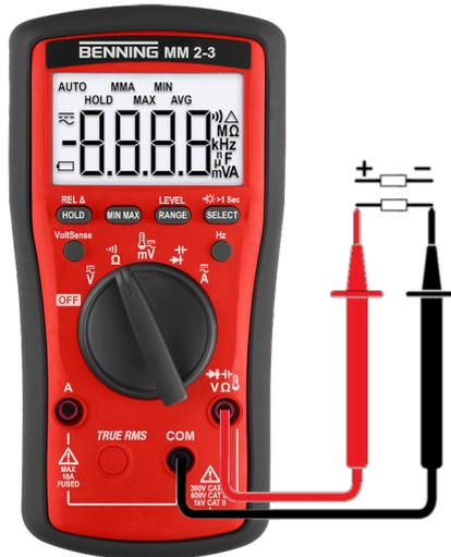
Figure 11: Resistance measurement or continuity test
