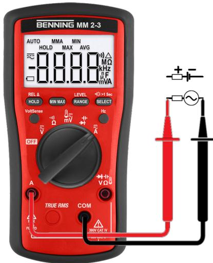
Figure 10: Current or frequency measurement
