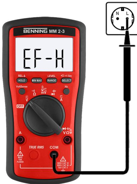
Figure 15: External conductor or phase testing
