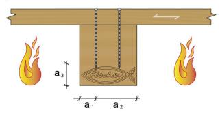
Figure N4.1: Fire design for axially loaded screws (figure not to scale)
