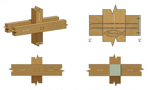
Figure N2.1: Fire design for protected screws – laterally loaded (figures not to scale)
