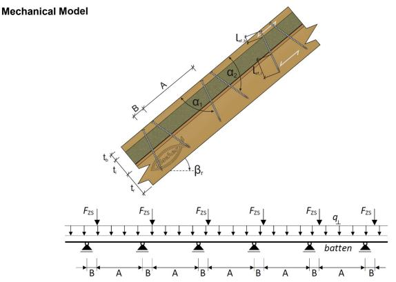
Figure L11.1: Counter batten on rafters with alternatively inclined screws and mechanical model (figure not to scale)
