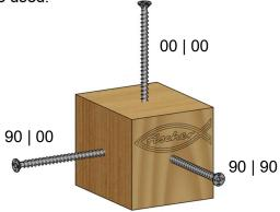
Figure D9.1: fischer PowerFull II in LVL-d (figure not to scale)
