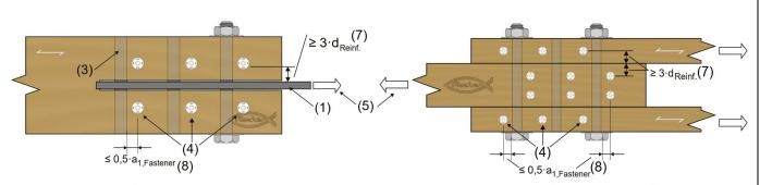
Figure J1.1: Shear connections with bolts - reinforcements with internal screws (figures not to scale)
