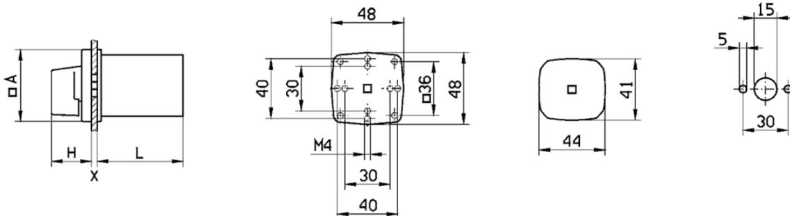
A= 48mm, H= 27mm, Xmax= 4mm, L= 69mm
